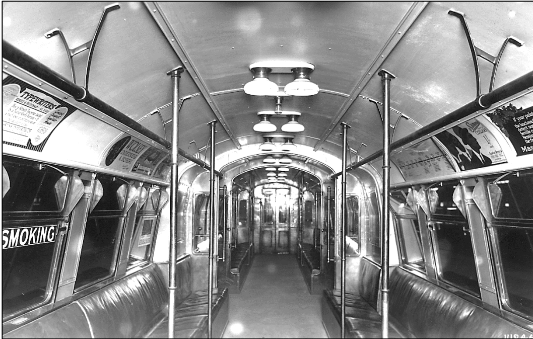
Figure 2: Interior of 1920 Cammell Laird stock car as built with plain leather longitudinal seating, vertical grab poles, horizontal handrails, plain cement flooring and twin, shaded lamps down the centre of the ceiling. The design was similar to the District Railway's F Stock of the same era. Both were later re-modelled with moquette seating and rearranged lighting.
