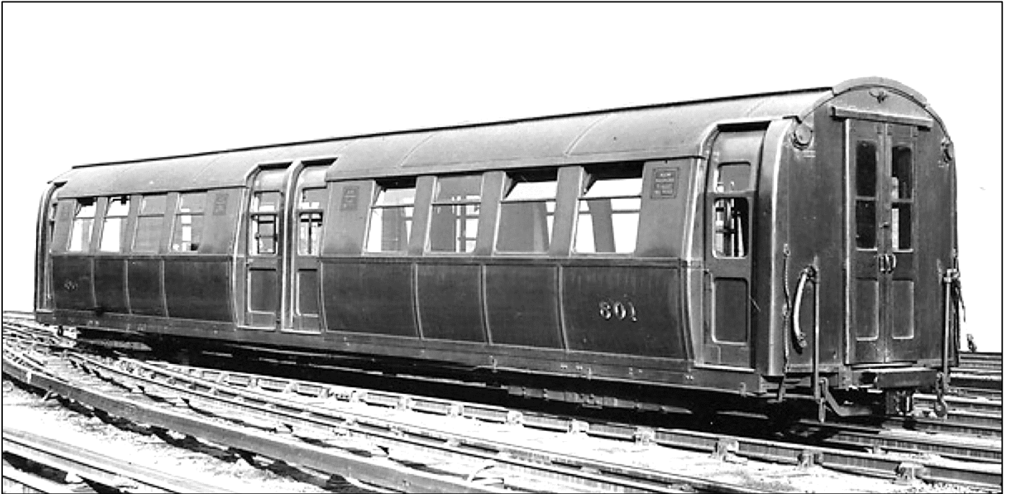
Figure 1: 1920 Cammell Laird Stock trailer car No. 801 as photographed in Lillie Bridge depot in February 1925, over four years after it was delivered. The curved bodyside shape was an attempt to make room for the “air engines”, as the door operating equipment was called, without reducing the seat and standing spaces too much. The central double door opening was strengthened by a substantial vertical pillar some 7 inches wide. The car end shows the sockets for the auxiliary and control jumpers on either side at roof level and, over the centre doorway, the socket for the emergency lighting jumper. These cars were not provided with heaters. Photo: LT Museum.
